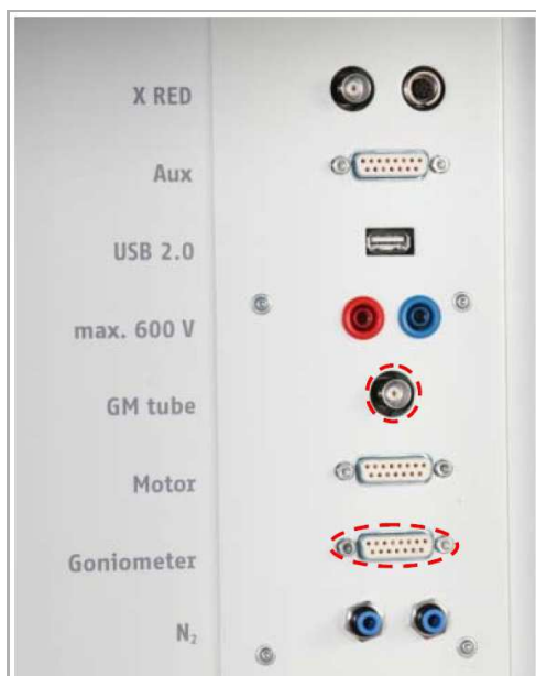
Fig. 2: Connectors in the experiment chamber
