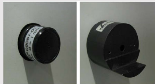
Fig. 4: Installation of diaphragm and crystal holder.
