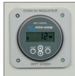
Controller screen attached to the side of the cabinet
