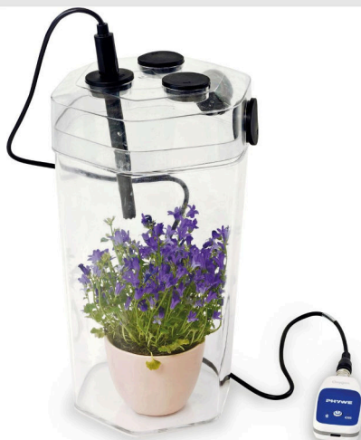
Experimental setup with reaction chamber, plant and oxygen sensor
