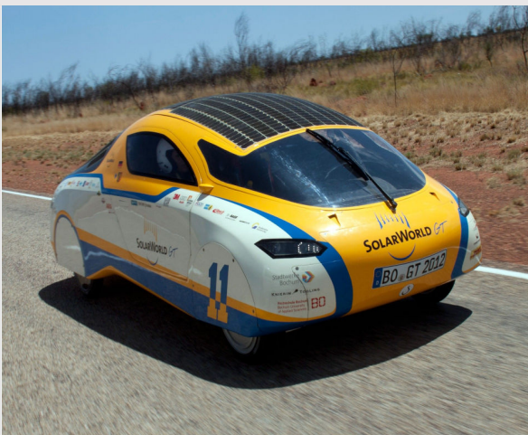
Solar cells on the roof of the SolarWorld GT experimental vehicle
