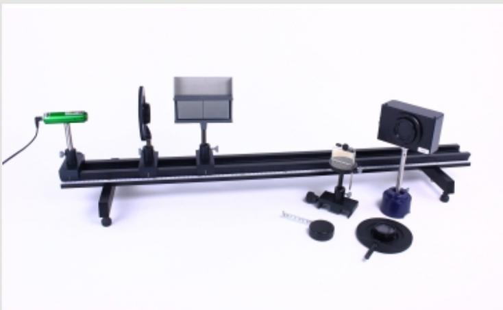
Experimental set-up for producing interference with the Fresnel mirror.
