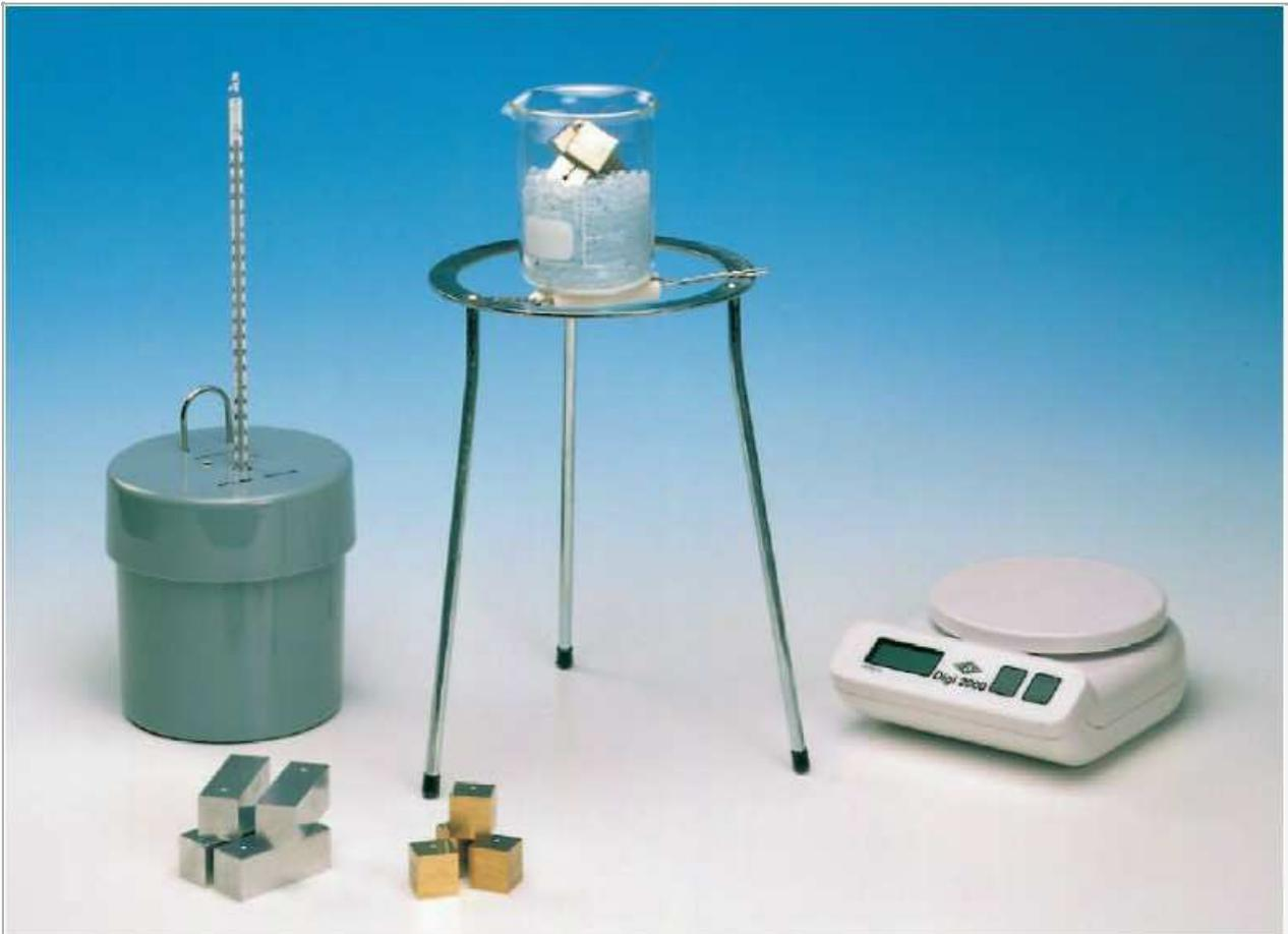
Fig. 1: Experimental set-up for determining the heat capacity of metals.
