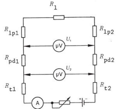
Fig. 3b: Equivalent circuit diagram:  $R_t$ ,  $R_{pd}$  and  $R_{1p}$  are contact resistors,  $R_1$  a line resistor.
