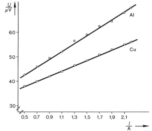
Fig. 2: Current/voltage characteristics of a copper rod and an aluminium rod.
