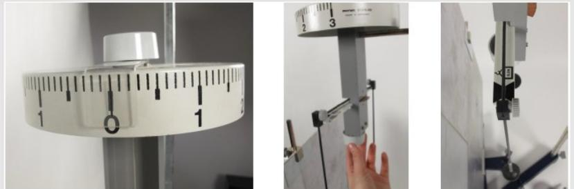
Fig. 5: Adjusting of the torsion dynamometer
