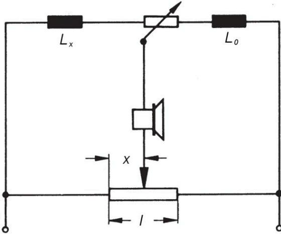
Fig. 4: Schematic circuit for task 2 (inductances).
