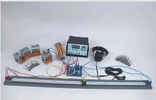
Fig. 1: Experimental set-up for determining unknown inductances
