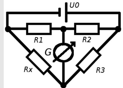
Fig. 2: Schematic circuit of the Wheatstone bridge
