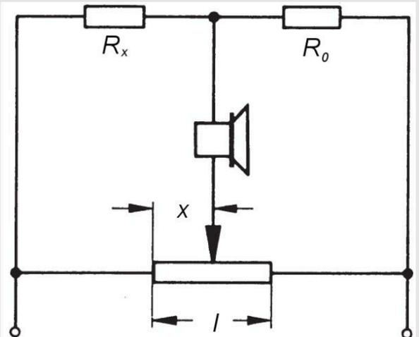
Fig. 3: Schematic circuit for task 1 (ohmic resistances).
