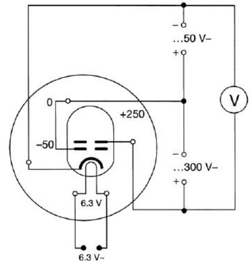
Wiring diagram for Narrow beam tube
