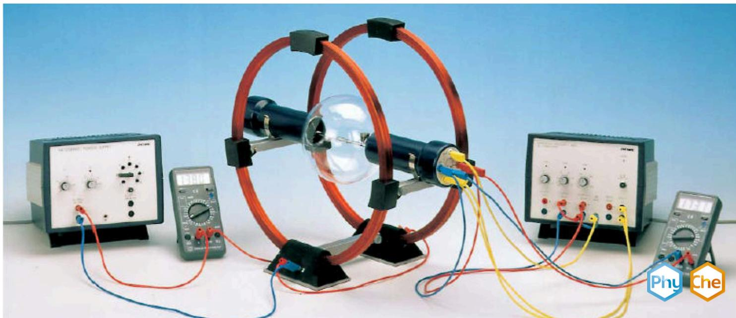
Electrons are accelerated in an electric field and enter a magnetic field at right angles to the direction of motion. The specific charge of the electron is determined from the accelerating voltage, the magnetic field strength and the radius of the electron orbit.
