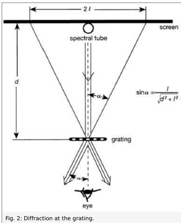
Fig. 2: Diffraction at the grating.
