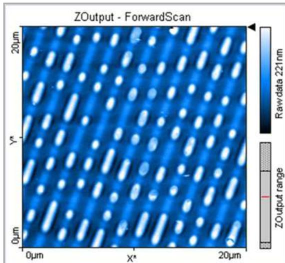
Figure 33: 20-µm Image of CD Stamper. Note that the curvature of the tracks is not discernible at this scan size.
