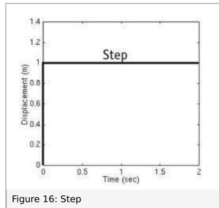
These three gains can be set individually and define how fast and in which manner the error is minimized and the therefore how good the topography of the sample is reproduced in the measurement. Thus it is important to understand its characteristics. To illustrate the effect of the PID gains consider the following experiment. A step signal from 0 to 1 will be measured (see *Figure 16: Step*).
