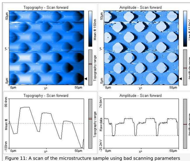
Figure 11: A scan of the microstructure sample using bad scanning parameters
