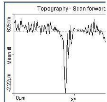
Figure 26: High Gain. Oscillating signal set too high.
