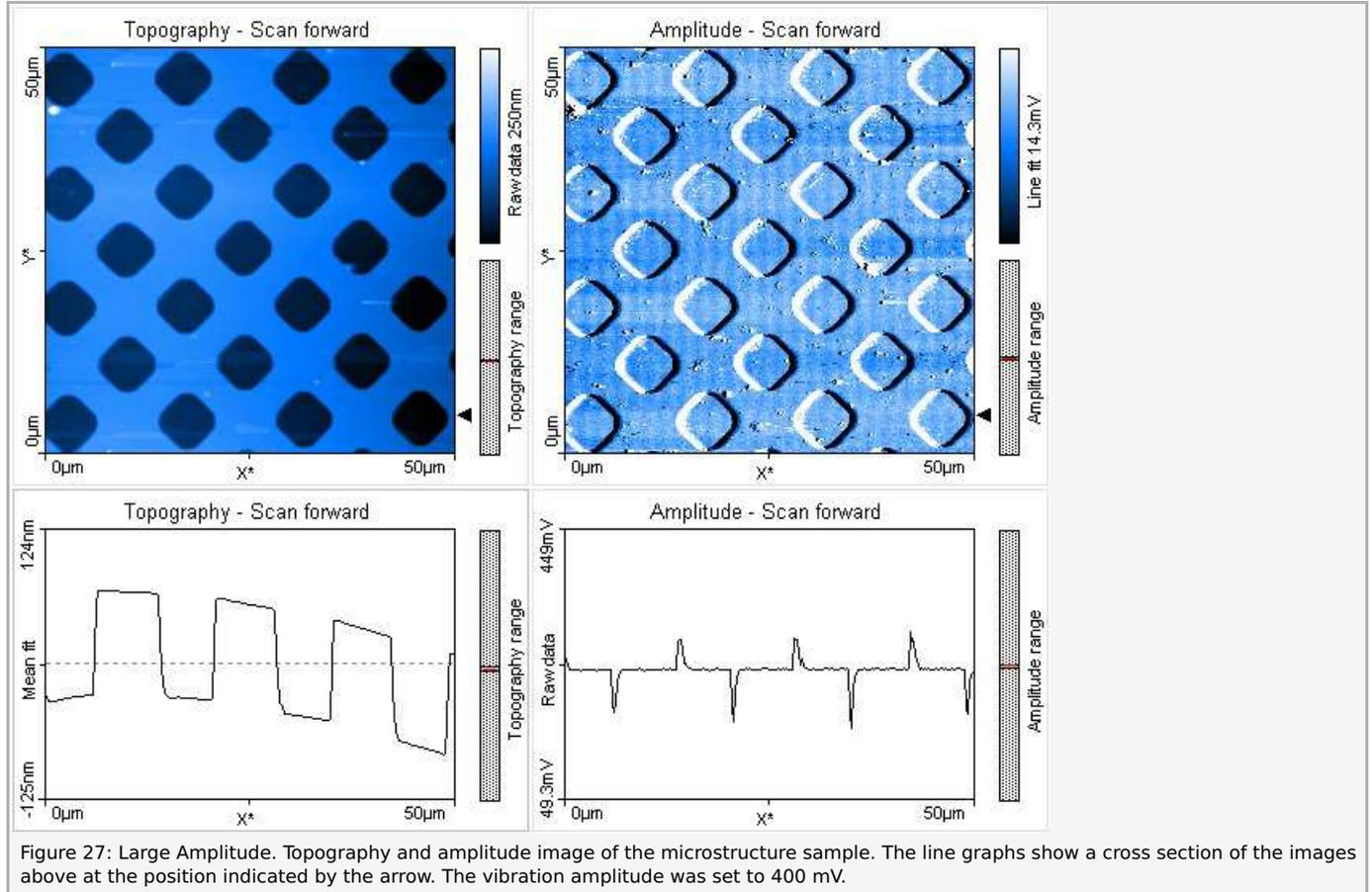
Figure 27: Large Amplitudeshows the topography and amplitude image of the microstructure sample. The line graphs show a cross section of the images above at the position indicated by the arrow at the right side of the sacn. It is clearly visible that the in the topography the slopes are steep. After each perturbation the amplitude signal is also corrected to the Set point value very quickly.
