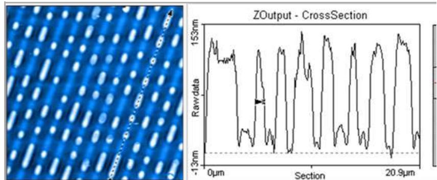
Figure 34: Bump length. Using the Measure Length tool in the track direction.
