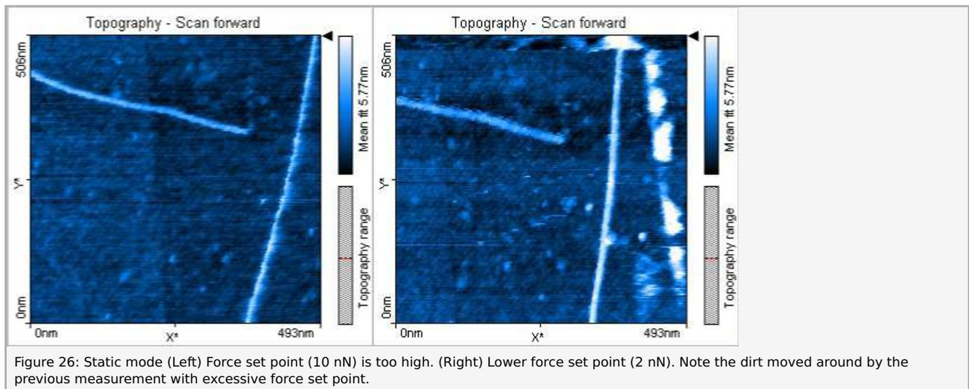
The investigation of the influence of the setpoint can be observed best when measuring the carbon nanotube sample in static mode using a suitable cantilever. This sample represents the group of materials with macromolecules that are used for molecular nanotechnology. Other well-known examples are self-assembled particles, DNA, and nanotubes made of other materials.
