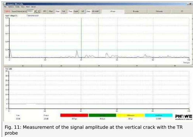
Fig. 11: Measurement of the signal amplitude at the vertical crack with the TR probe
