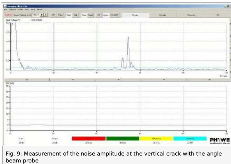
Fig. 9: Measurement of the noise amplitude at the vertical crack with the angle beam probe
