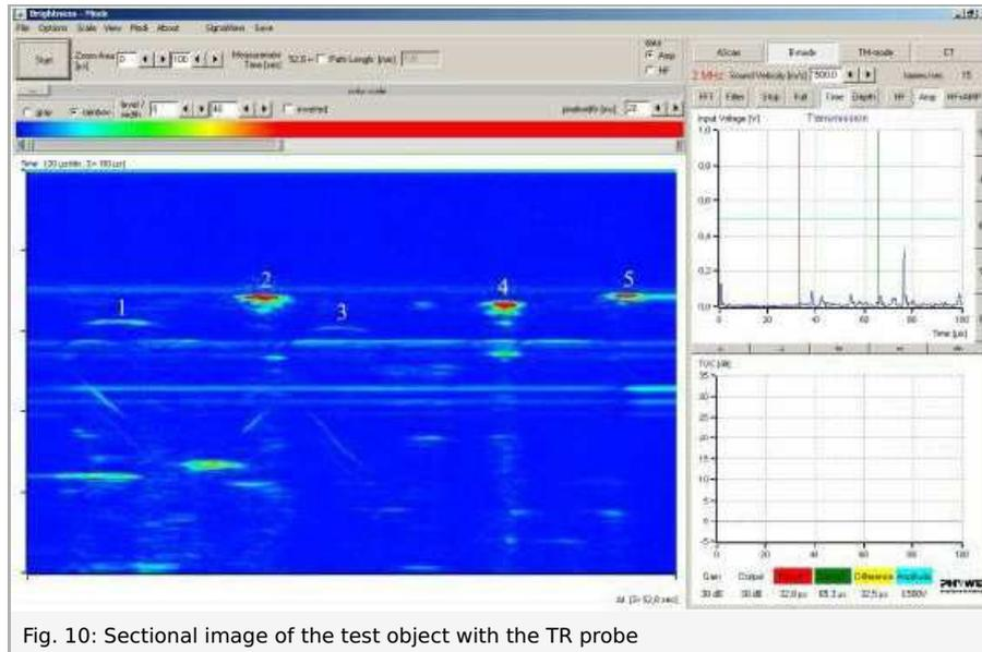
Fig. 10: Sectional image of the test object with the TR probe
