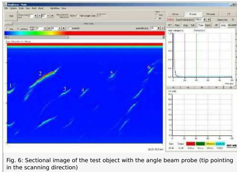
Fig. 6: Sectional image of the test object with the angle beam probe (tip pointing in the scanning direction)
