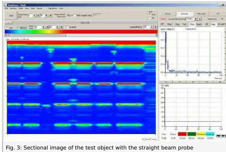
Fig. 3: Sectional image of the test object with the straight beam probe
