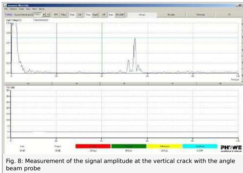
Fig. 8: Measurement of the signal amplitude at the vertical crack with the angle beam probe
