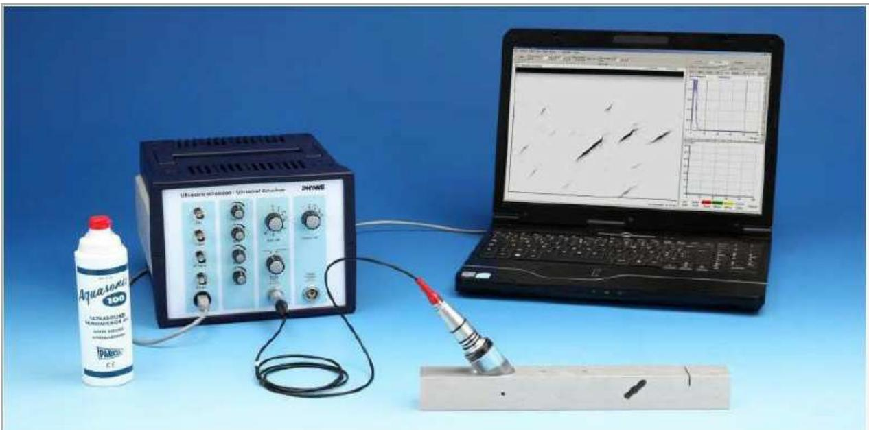
Fig. 1: Detection of discontinuities: experimental set-up
