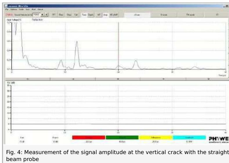
Fig. 4: Measurement of the signal amplitude at the vertical crack with the straight beam probe
