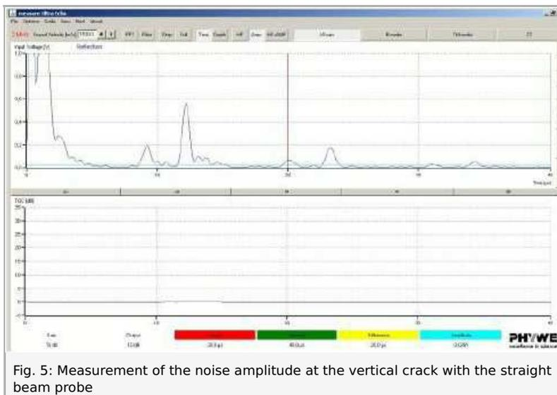
Fig. 5: Measurement of the noise amplitude at the vertical crack with the straight beam probe
