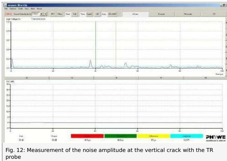
Fig. 12: Measurement of the noise amplitude at the vertical crack with the TR probe
