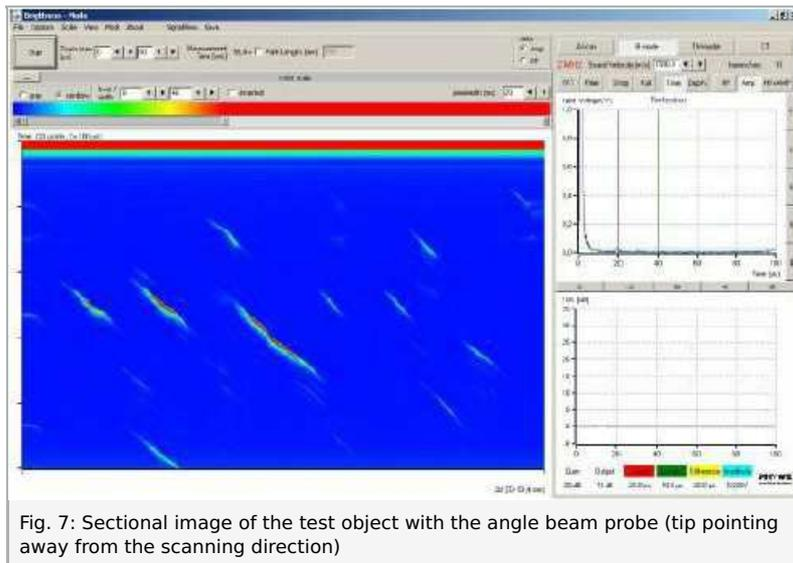
Fig. 7: Sectional image of the test object with the angle beam probe (tip pointing away from the scanning direction)
