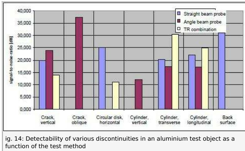
Vertical cylinders are the most difficult to detect, since only the small corner echoes at the bottom of the test object can be captured with the angle beam probe.
