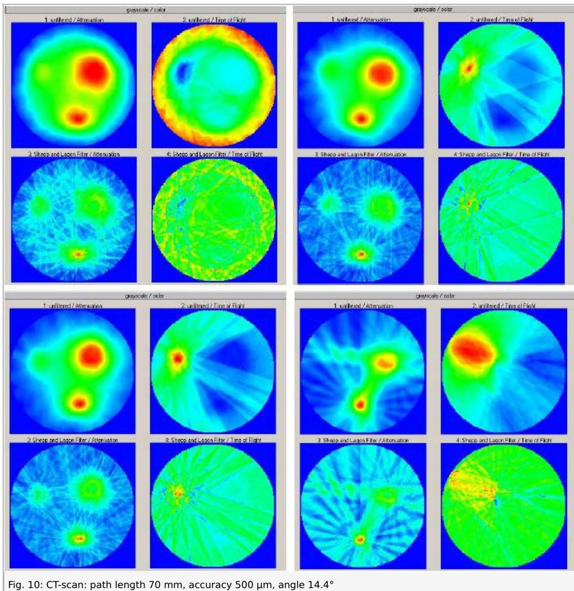
Fig. 10: CT-scan: path length 70 mm, accuracy 500  $\mu$ m, angle 14.4°
