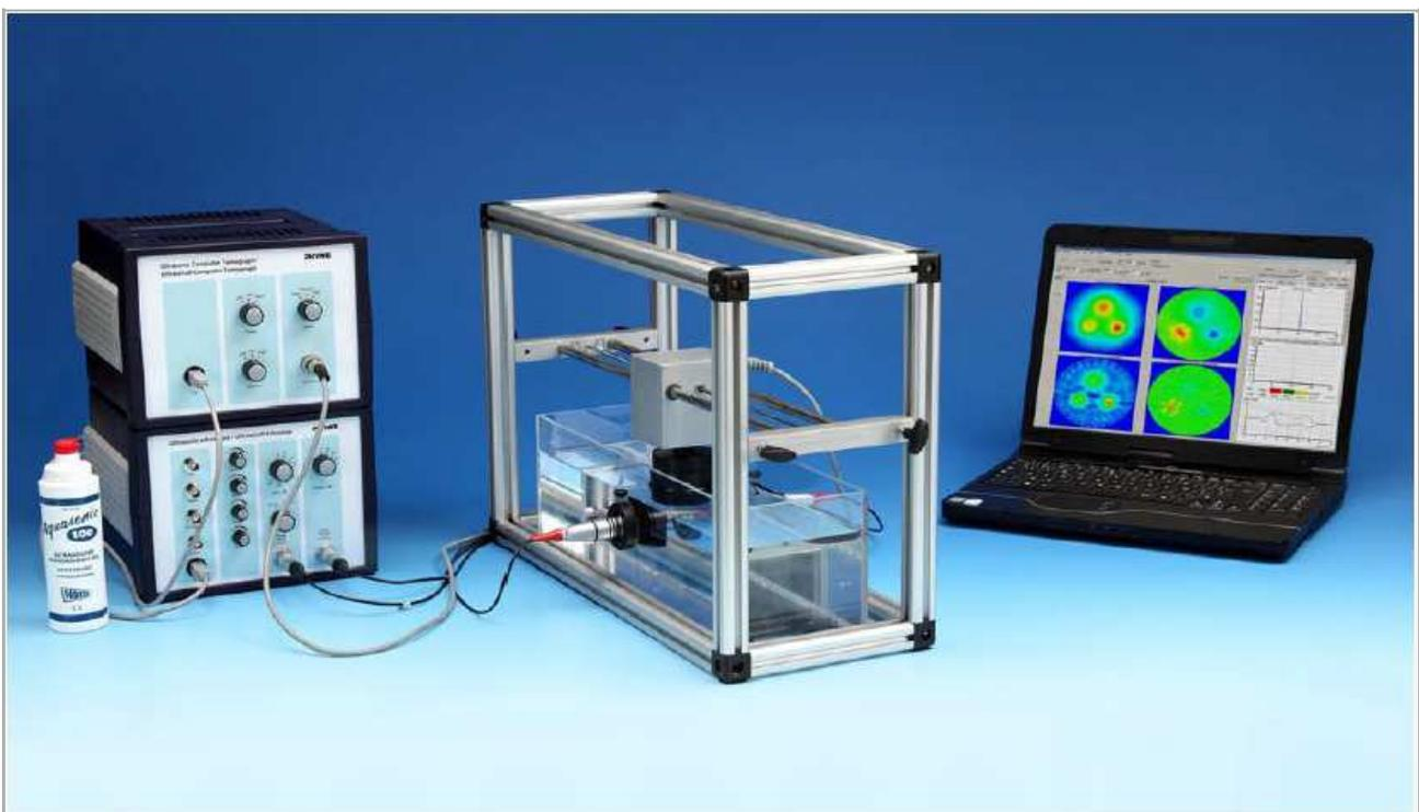
Fig. 1: Equipment for ultrasound computed tomography, experimental set-up
