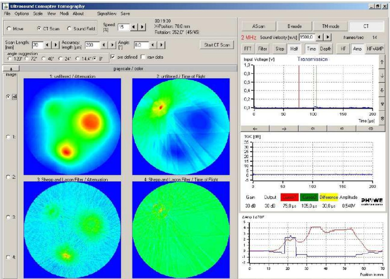
Fig. 9: CT-scan: output 30 dB, gain 30 dB, path length 70 mm, accuracy 200 µm, angle 8°
