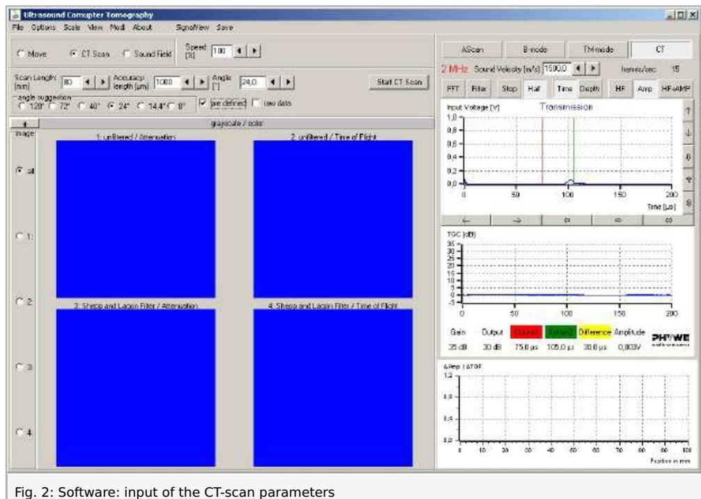
Fig. 2: Software: input of the CT-scan parameters
