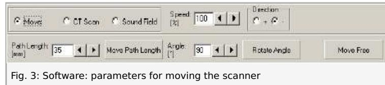
Fig. 3: Software: parameters for moving the scanner
